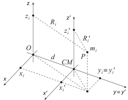
$$\begin{aligned} I &= \sum_i m_i (x_i^2 + y_i^2) = \sum_i m_i [x_i'^2 + (y_i' + d)^2] = \sum_i m_i (x_i'^2 + y_i'^2 + 2y_i'd + d^2) = \\ &= \sum_i m_i (x_i'^2 + y_i'^2) + 2d \sum_i m_i y_i' + d^2 \sum_i m_i. \end{aligned}$$
