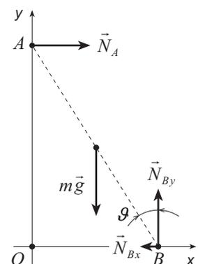
$$\vec{r}_{mg} \times (m\vec{g}) - \vec{r}_{F_A} \times \vec{N}_A = \vec{0}$$
