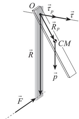
$$\vec{\mathcal{I}}_\tau = \int_{t_1}^{t_2} \vec{\tau} dt = \int_{t_1}^{t_2} (\vec{R} \times \vec{F}) dt = \vec{R} \times \int_{t_1}^{t_2} \vec{F} dt = \vec{R} \times \vec{\mathcal{I}},$$
