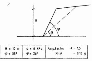
FIG. 3. Schematic Representation of Studied Slope
