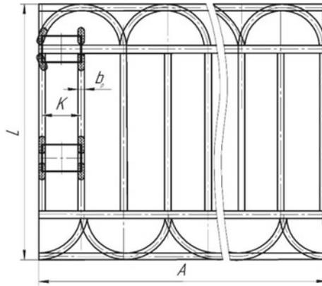
**Fig. 3** Scheme of field map planning for the track system of agriculture for the operation of the bridge tractor
