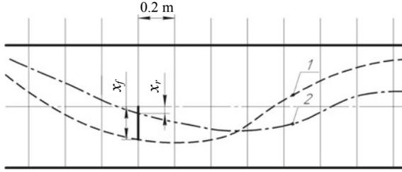
**Fig. 2** Scheme for determining the transverse displacement of the bridge tractor: 1, 2 – respectively, the middle of the trajectories of its front and rear wheels within the width of the technological track
