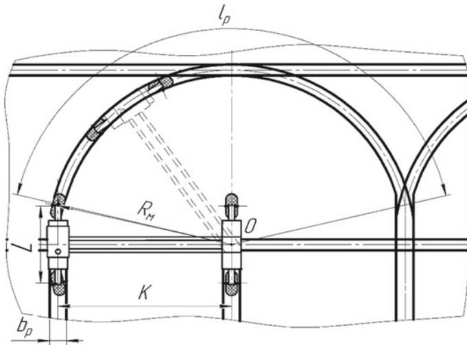
**Fig. 4** Diagram of the rotation of the bridge tractor by its circular rotation relative to the center of rotation (point O)
